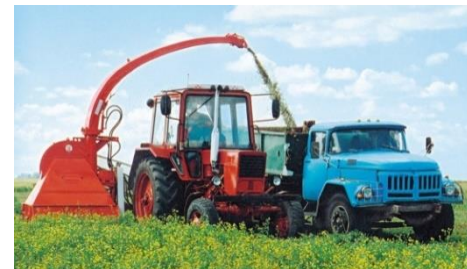
CH15 Mounted rotary mower-shredder Required power 55 h.p. Operating speed 8 km/h Operating width 1,5 m Discharge height 3,6 m
