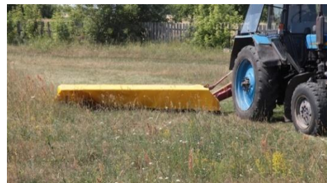
TRAVERS 280M Mounted rotary mower Required power 80 h.p. Operating speed 12 km/h Operating width 2,8 m Swath width 2,5 m
