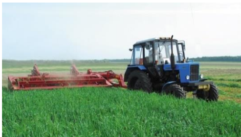
CT42 Pull-type mower-conditioner Required power 80 h.p. Operating speed 7 km/h Operating width 4,2 m Swath width 0,8-1,6 m
