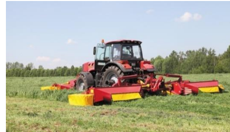
TRAVERS 870M Mounted rotary mower-crusher Required power 218 h.p. Operating width 8,7 m Quantity of disks 8 pcs Swath width 1,8 m
